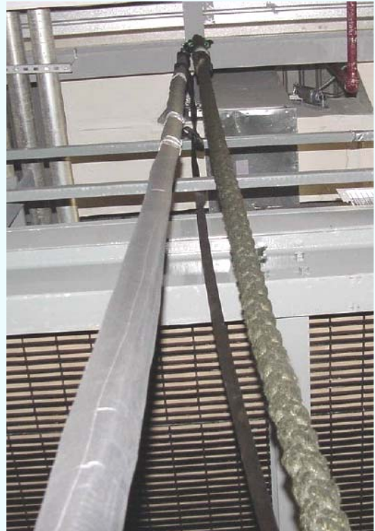
Figure 3. Radially compressive rope hanging next to a standard climbing rope.
