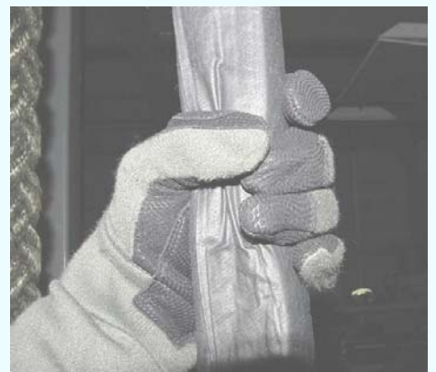
Figure 2. Squeezing by hand compresses rope minimizing need of friction.
