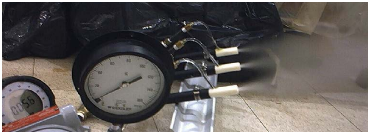
Figure 1. Three nozzles in parallel generating very fine mist with very low pressure gas.
