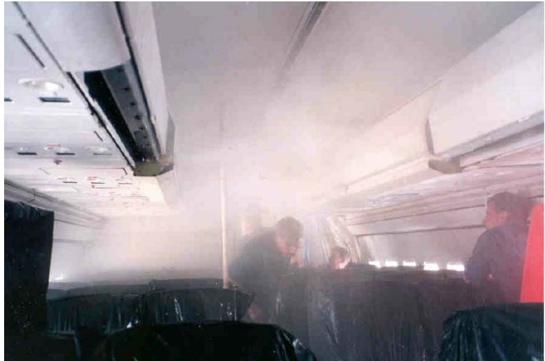
Figure 2. Fire Extinguishing Test of Nozzle System in Aircraft Compartment
